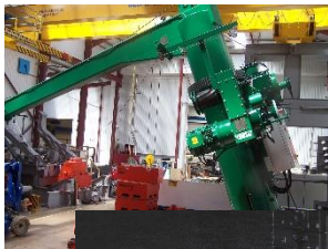
Welin Lambie Type: SARBE 8 C all electric rescue boat davit designed for tug applications
